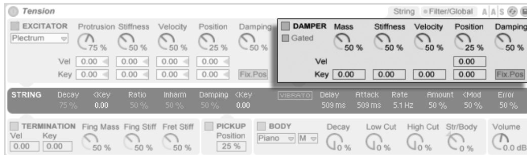
Tension's Damper Section.
